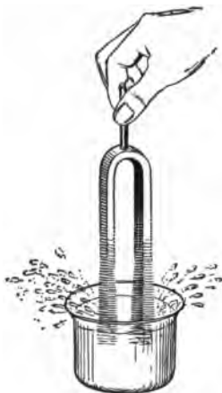
FIG. 145. — Sprays of water show that the fork is in motion.
